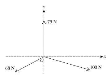
Three coplanar forces of magnitudes 68 N, 75 N and 100 N act at an origin O, as shown in the diagram. The components of the three forces in the positive x-direction are -60 N, 0 N and 96 N, respectively. Find
